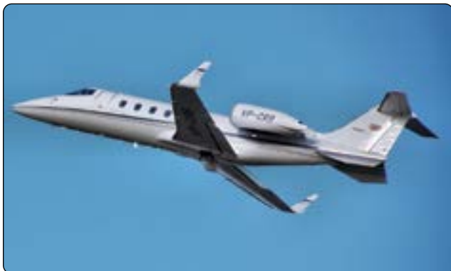
Figure 2-17. Winglets on a Bombardier Learjet 60.
